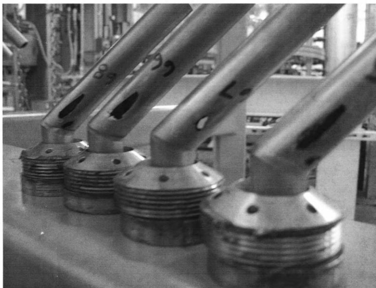
Pulse Jet Mixers show gaping holes after only five tests. Will they really last for 40 years without maintenance? Click here for a higher resolution image.
